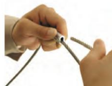
3. Loop the Wire Rope from Eyelet
