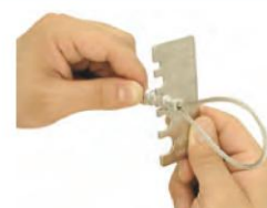
QUALITY CHECK SLEEVE WITH GAUGE, PASS THROUGH SWAGING COMPLETE!
