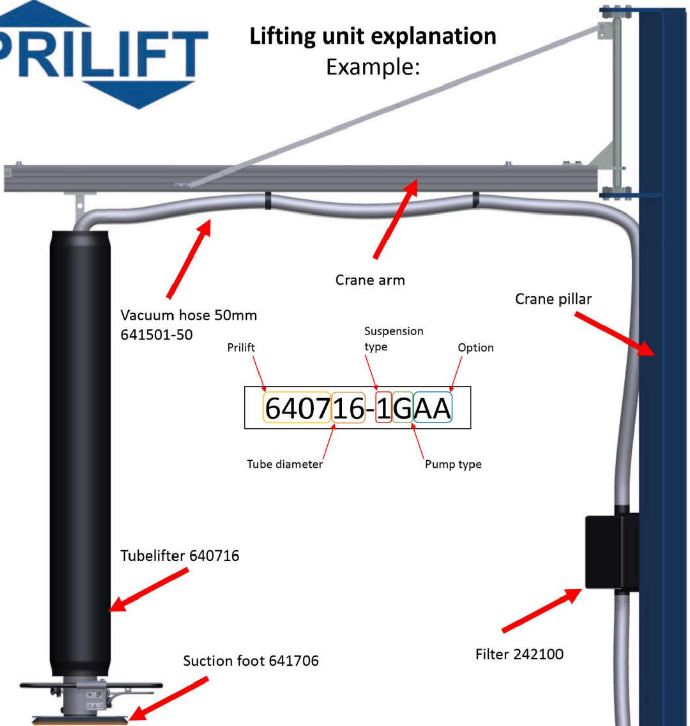
Lifting unit = Tube lifter + Vacuum pump
